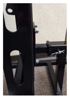
Carrier inserted and secured into receiver
