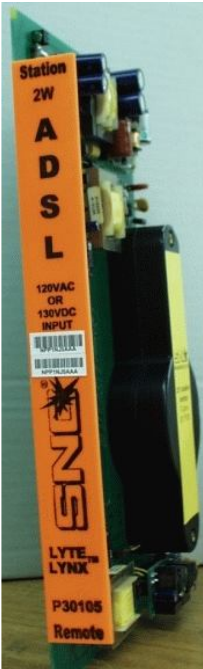
Figure 1: ADSL Isolation Cards
